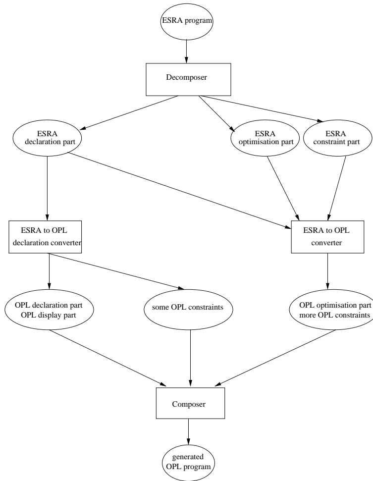
Fig. 4. Architecture of the ESRA compiler
