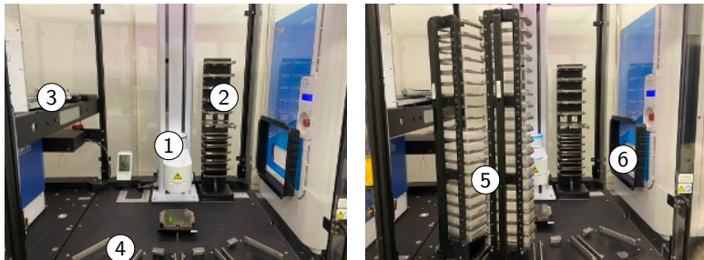
Figure: 1) the robotic arm, 2) the plate delidder, 3) the sealer, 4) base for plate hotels, 5) plate hotels, 6) the dispenser.
